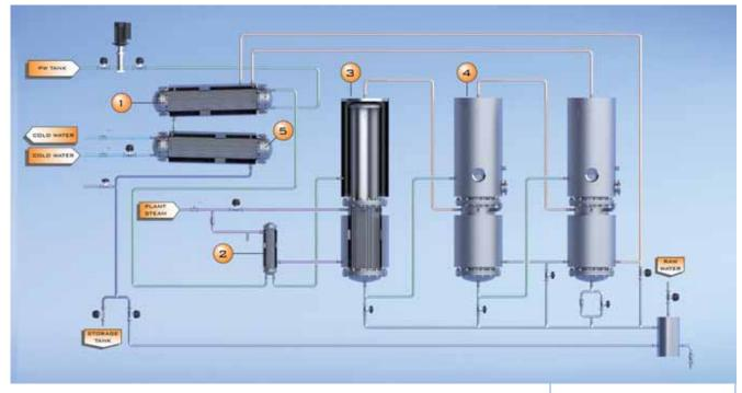
Feed water (PW) is pre-heated by means of two DTS heat exchangers, which use respectively the heat of the pure steam and distillate water outlet and the plant steam outlet. The first column of the CS water still is equal to our CPS steam generators, heated also with plant steam.
